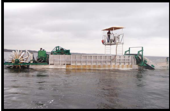
Mechanical harvester that has been modified to harvest hydrilla in deep water
